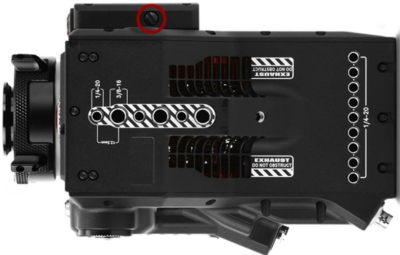
Figure: Focus Hook Screw Storage Location
