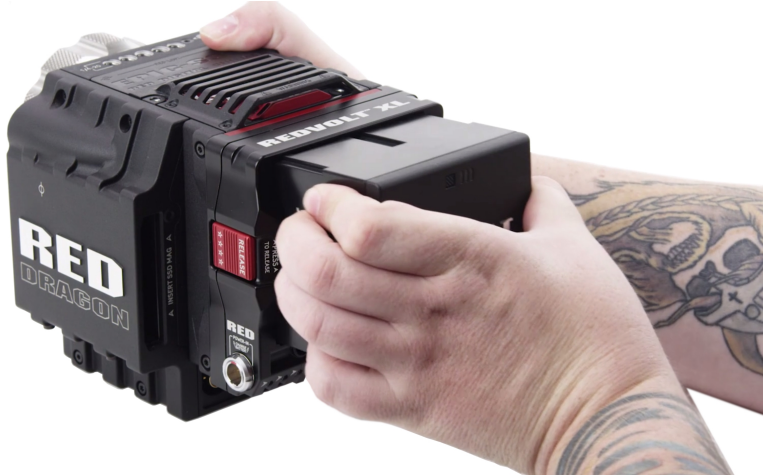
Figure: Insert a REDVOLT XL Battery
