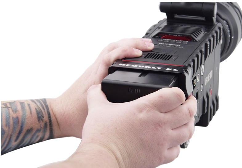
Figure: Remove a REDVOLT XL Battery
