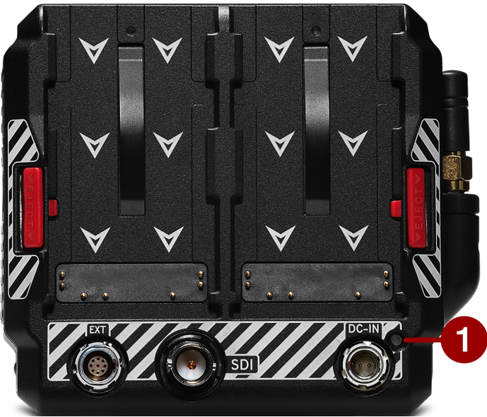
Figure: KOMODO 6K, DC/Battery LED
