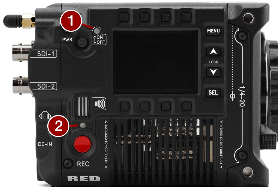
Figure: Camera LEDs, Right Side
