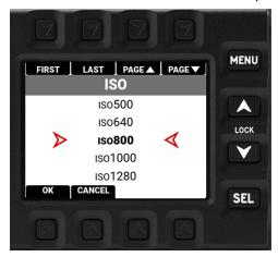
Press the buttons above FIRST, LAST, PAGE▲, or PAGE▼ or press the up or down arrow to navigate the list. Press SEL, or the button under OK, to select the item. Press MENU, or the button under CANCEL, to return to the menu without making a selection.
