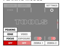
The Peaking tools are modes that provide different ways to indicate image focus. The Peaking modes you can select include:
