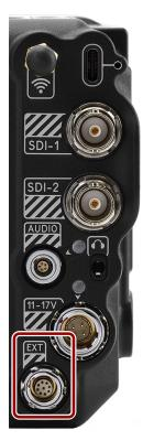
The female 9-contact 0B ODU Extension port supports serial (RS-232 RX and TX), a General Purpose Input (GPI) trigger (active-low switch closure), General Purpose Output (GPO), Timecode, and Genlock. The connector also offers auxiliary 5 Volt power out, with a maximum sustained current draw of 500 mA.
