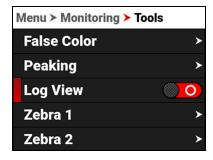
Press SEL to toggle the Log View switch between Enabled and Disabled:
