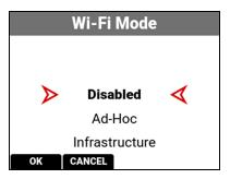
From Mode you can disable the Wi-Fi network, or you can enable the camera's Ad-Hoc or Infrastructure Wi-Fi settings. The default setting is Disabled.
