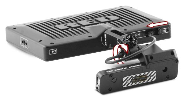
NOTE: The USB-C-style DSMC3 RMI cable is a custom-pinned cable, which is not compatible with standard USB-C cable ports.
