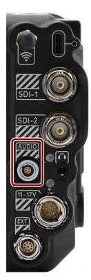
The female 5-pin 00B audio connector accepts 2-channel audio, Line, Mic, and +48V Phantom Power.
