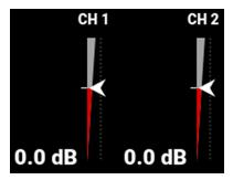
The audio level indicators move up and down to indicate the changes in the audio level adjustments. The level measured in decibels is displayed below the level indicators. You can adjust channels 1 and 2 individually, or you can link the channels and adjust them together.
