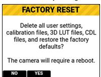
**NOTE:** Resetting the camera will delete all of your settings and remove all imported files. The camera turns off, and then back on to complete the reset process.
