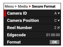
2. From the Secure Format menu, select the desired Camera ID, Camera Position, Reel Number and Edgecode. Navigate down to the Format button and press SEL to start the Secure Format process:
