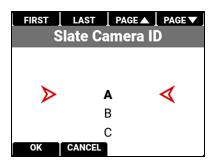
The camera IDs you can assign when recording a clip include the letters A-Z.
