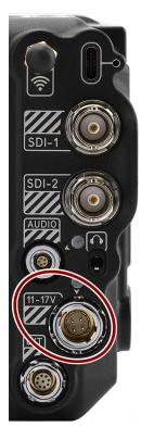
The male 6-Pin 1B DC-IN connector accepts DC input power from 11 V DC to 17 V DC. A built-in power conditioner protects against reverse-polarity connections, electrostatic discharge (ESD), undervoltage, overvoltage, and overcurrent.
