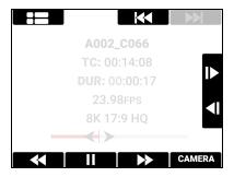
With the Playback screen buttons you can view the Clip list, move to the start of the clip, fast reverse, play/pause, fast forward, and move forward and reverse by a single frame.
