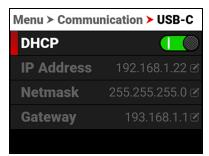
When DHCP is not enabled, you can select IP Address and manually enter a static IP address.
