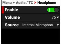
You can enable and disable the headphone audio jack by pressing SEL to toggle Enable to the right (green / enabled) and to the left (red / disabled).
