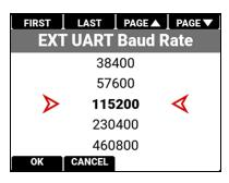
The Baud rate controls how fast data is transmitted over the serial connection. The higher the speed, the more likely that errors can occur. The Baud rates you can choose include:
