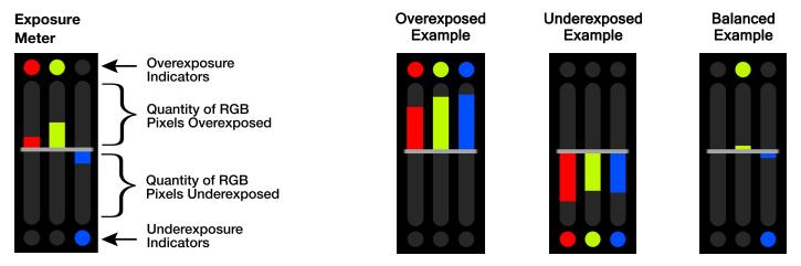
RGB Exposure Meter displays the quantity of over or under exposed pixels in each of the separate red, green, and blue channels.
