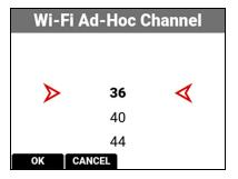
Select the optimal channel for the selected band, one which receives the least interference from the surrounding Wi-Fi signals.
