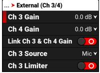
The External audio is represented as Channels 3 and 4 on the Home Page and on the Audio Channels 3/4 Page VU Meters (refer to LCD for more information). The left channel is channel 3 and the right channel is channel 4.
