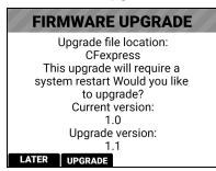
9. Press the button under UPGRADE to confirm. The Firmware Upgrade progress screen displays:
