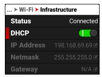
When DHCP is not enabled, you can manually enter a Netmask address. This screen opens automatically after you enter a static IP address.
