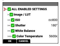
Press the button under OK to create the preset. The Preset Name screen opens.
