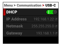
When DHCP is not enabled, you can select Netmask and manually enter a Netmask address. This screen opens automatically after you enter a static IP address.
