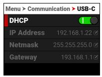
When DHCP is not enabled, you can select Gateway and manually enter a Gateway address.
