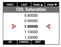
The CDL Saturation settings range from 0.00000 to 4.00000. The default CDL Saturation setting is 1.00000.
