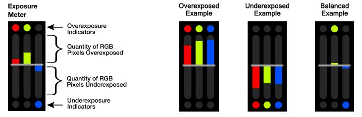
RGB Exposure Meter displays the quantity of over or under exposed pixels in each of the separate red, green, and blue channels.
