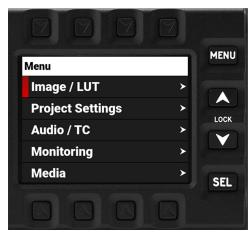
Press the up and down arrows to navigate up and down in the menu list. Press SEL to select a menu and open the submenus:
