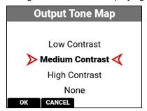
When shooting in R3D format, the camera stores this as metadata, which you can adjust non-destructively in post production after filming.
