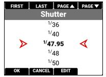
You can switch between angle and time by using the Status Settings or by pressing and holding the button above SHUTTER on the Home Page (refer to Home Page).
