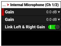
The Internal Microphone is represented as Channels 1 and 2 on the Home Page and on the Audio Channels 1/2 Page VU Meters (refer to LCD for more information). The left channel is channel 1 and the right channel is channel 2.
