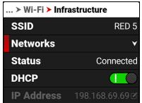
When a network is selected, the SSID displays the Wi-Fi network name (SSID).
