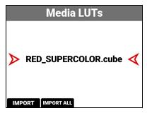
3D LUTs can be imported from media to the camera. When importing 3D LUTs from media to the camera, the 3D LUTs must be saved on the root path of your media, in a folder titled "luts."
