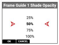
Use Shade Opacity to select the percentage of opacity for the shading outside of the Frame Guide:
