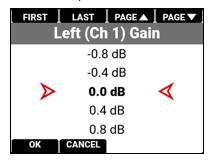
You can adjust the internal audio levels for left and right from -52.5 dB to 36.0 dB.
