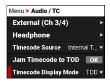
3. Press SEL to select Timecode Display Mode. The Timecode Display Mode menu opens:
