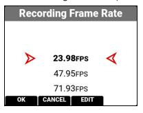
The recording frame rate is the number of frames per second (FPS) that are recorded. The recording frame rate is different from the project time base, which is the rate at which the footage will be played back.
