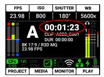
**NOTE:** Each new media card will default to an edgecode track starting at 01:00:00. You can change the edgecode to begin at any desired time by using the Media Format menu (refer to Edgecode).
