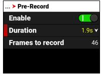
Pre-Record allows you to continually capture images to a small amount of memory while waiting to begin recording. This allows you to capture unexpected events such as, a whale breaching the water, or a an athlete scoring a goal. When you finish recording, the pre-recorded clip is added to the beginning of the recording.
