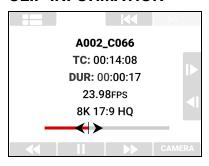
The Clip Information displays the name, Timecode, duration, project time base, format, and timeline of the clip.
