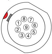
Figure: Front face of the female 9-contact Extension port (looking at the back of the camera).
