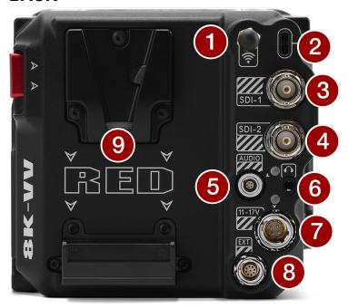
Figure: Camera Body Rear Controls and Features
