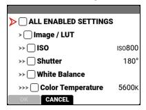
You can also use the ALL ENABLED SETTINGS checkmark button to select all of the current camera settings as a preset:
