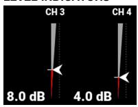
The audio level indicators move up and down to indicate the changes in the audio level adjustments. The level measured in decibels is displayed below the level indicators. You can adjust channels 3 and 4 individually, or you can link the channels and adjust them together.
