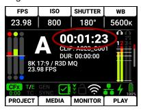
This text turns red when the camera is recording.
