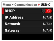
When connected to an Ethernet network, this allows you to enable or disable Dynamic Host Configuration Protocol (DHCP).
