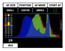
The LCD Histogram page is the second page on the LCD. Press the down button to navigate from the Home page to the Histogram page.
