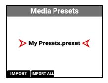
You can import presets from the media to the camera. When importing presets from the media to the camera, the presets are saved to a folder on the camera called "presets."
