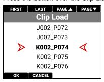
Navigate to the desired clip and press the button under OK to open the clip in the Playback screen.
