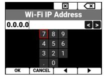
After you enter the static IP address, the Netmask entry screen opens.
