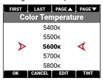
When the image's light source color temperature is warm, you can compensate by setting the camera to a warmer color temperature. When the image's light source color temperature is cool, you can compensate by setting the camera to a cooler temperature.
