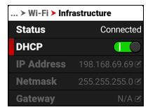
When DHCP is not enabled, you can manually enter a static IP address.
