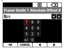
Use the keypad to enter the number of pixels for X/Y offset and for the width and height of the Frame Guide. The Absolute items are only enabled when you select Absolute Mode.
