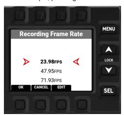
Press the up and down arrows to navigate the list. Press the button below OK or press the SEL button to accept the choice and return to the Home Page. Press the button below CANCEL or press the MENU button to return to the Home Page without making a change. Press the button under EDIT to open a manual editing screen.
