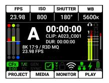
This section describes the Home Page of the LCD GUI. This page contains the Quick Settings, Exposure Meter, Recording Information, VU Meter, Status Bar, and Quick Menus. This is the first page that displays when you power up the camera.
