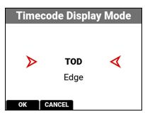
Select Edge and press the button under OK to use Edgecode. The camera displays the Edgecode on the LCD Home page:
