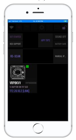
The camera icon displays the camera's Ethernet IP address:
