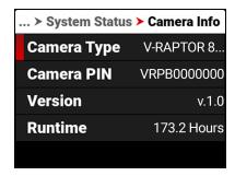
Version displays the currently installed camera firmware. A higher number reflects a newer release.
