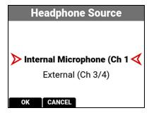
You can select the internal microphone channels 1 and 2, or you can select the external channels 3 and 4.
