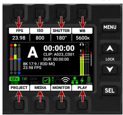
In this example, pressing the button above FPS opens the Recording Frame Rate selection list:
