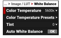
When shooting in R3D format, the camera stores white balance as metadata, which you can adjust non-destructively in post production after filming.
