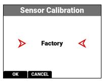
You should always select User calibration. The first time you calibrate the camera, the only choice is Factory. After you perform a calibration, the User calibration profile is added to the list and the camera makes it the default calibration. Every time you calibrate the camera, the User profile is updated. The only time the User profile is removed, is when you perform a Factory Reset.
