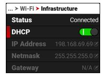
When DHCP is not enabled, you can manually enter a Gateway address.
