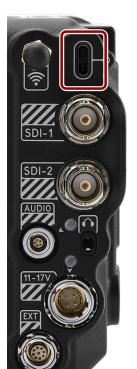
The USB-C power out connector supplies 5 Volts of power. The maximum sustained current draw is 0.5 Amps. The USB-C port is used primarily for data connections.
