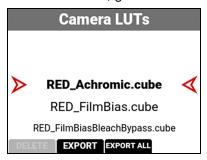
You can export 3D LUTs stored on the camera, to media, to use on other cameras. When you export 3D LUTs from the camera to media, the 3D LUTs are saved to a folder on the media called "luts."
