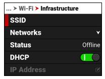
Use the Infrastructure menu to configure the Wi-Fi settings to connect to an existing Wi-Fi infrastructure:
