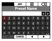
Use the Preset Name screen to name the preset. When the name already exists in the camera, the name is highlighted in red and the OK option is grayed out:
