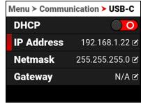
After you enter the static IP address and select OK, the Netmask entry screen opens.
