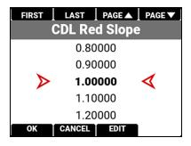
The CDL Slope settings range from 0.00000 to 2.00000. The default CDL Slope setting for each color is 1.00000.
