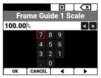
Use the keypad to enter the percentage of the image the Frame Guide contains.
