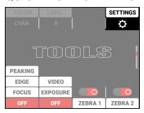
Press the button above SETTINGS to open the Quick Monitoring Menu.
