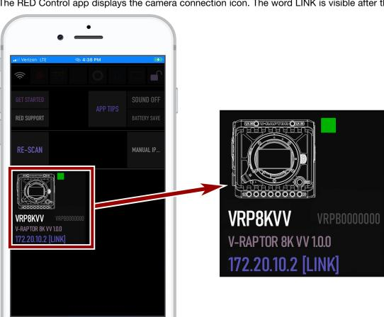
The RED Control app displays the camera connection icon. The word LINK is visible after the IP address.
