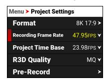
A Recording Frame Rate highlighted in Vellow will result in playback occurring at a different frame rate than the original recording, and will record varispeed audio.
