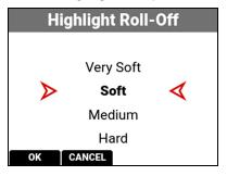
When shooting in R3D format, the camera stores this as metadata, which you can adjust non-destructively in post production after filming.
