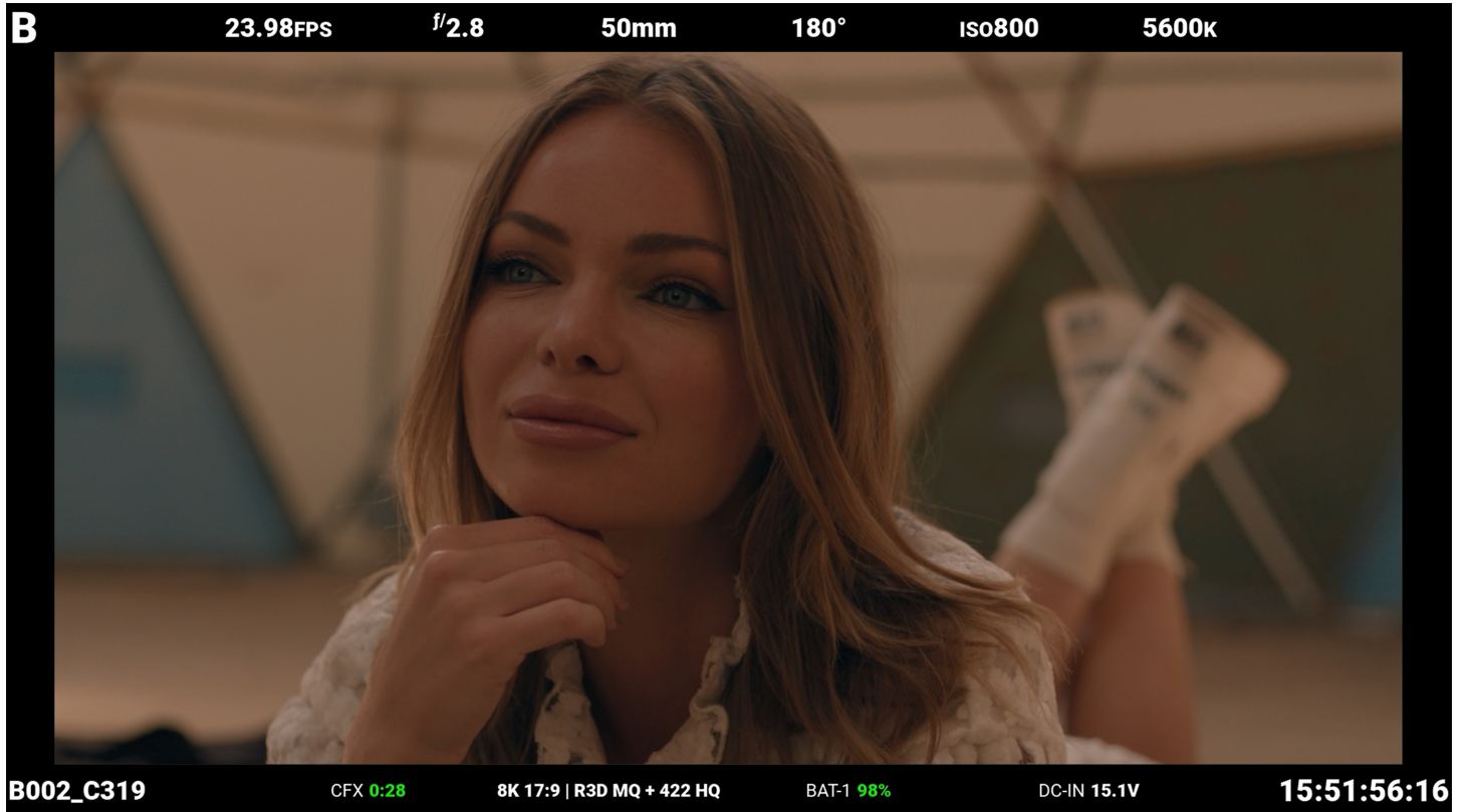
Figure: SDI monitor with SDI Standard Overlay Mode enabled
