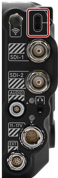
Figure: Front face of the USB-C port (looking at the back of the camera).
