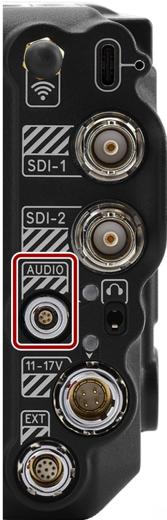
Figure: Front face of the female 5-Pin 00B audio connector (looking at the back of the camera).
